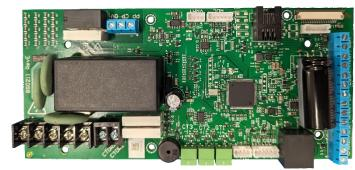
EEL is a fully-compliant 61851 AC charge controller that has all the necessary interfaces for any single or 3-phase AC charge solution.
